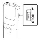
Slide the HOLD switch in the opposite direction from that of the arrow. The IC recorder is turned on, and "ACCESS" flashes.
